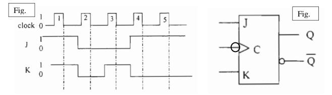
5. (b). (ii). For the positive edge triggered J-K flip flop with preset and clear inputs in the Figure below, determine the Q output for the inputs shown in the timing diagram if Q is initially LOW.
